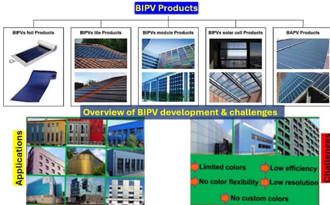
Figure 1. Examples of BIPV products, remaining challenges, and real-world applications of colored BIPV technologies, highlighting limitations in color diversity, efficiency, and resolution, as well as integration in modern facades (Basher et al., 2023; Basher & Basher, 2023).
